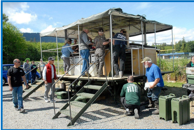
Joyce Emergency Management and Prep (JEPP) setting up It's MARK 99 MKT field kitchen. The kitchen is capable of feeding 300 people per day at the shelter.
